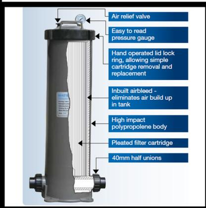
*Trimline cartridge filters utilise a specially treated synthetic fabric which is pleated into a cartridge. Cartridge filters are ideal for applications where backwashing may not be practical.*
